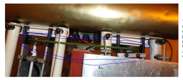
Top view existing drive pulleys on mine. You can just see the pulley below on the new drive. Just slide it to align
